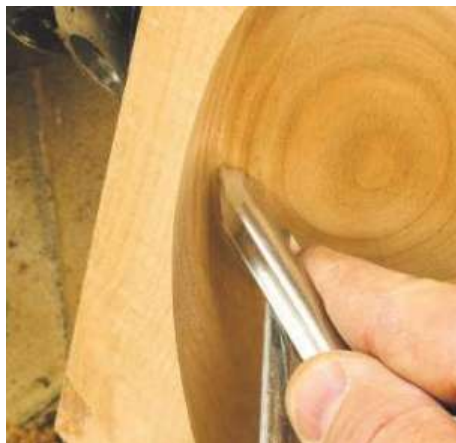
▲ Pic.17 I like to have a sharp punctuation point between the transitions of the shape. To get in this tight spot I changed to my signature gouge, which has a sharper bevel angle of around 40°
